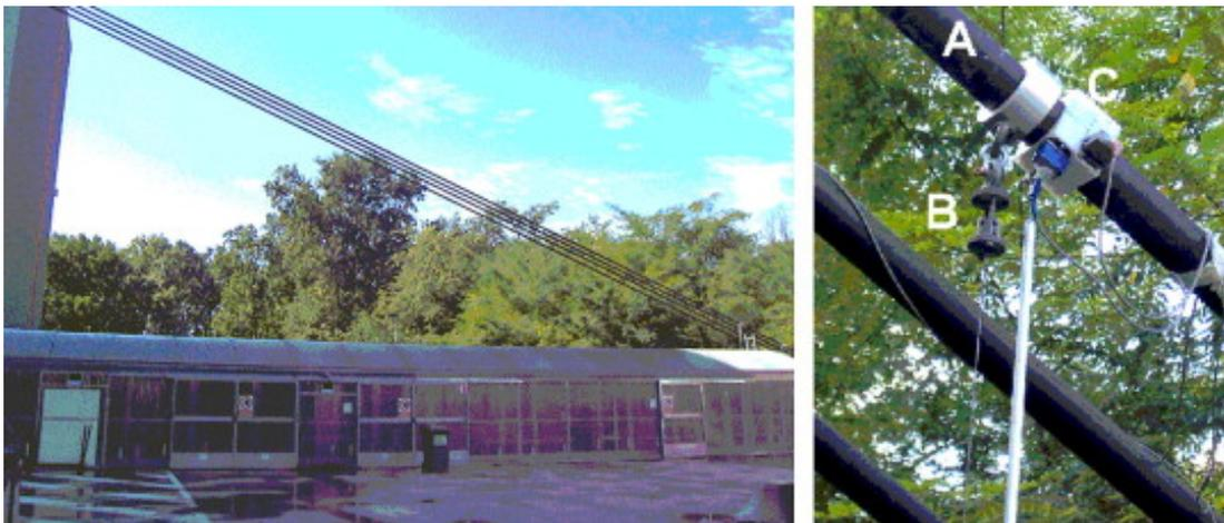
Figure 1.18: Four cables of 45 m long in ELSA (European Laboratory for Structural Assessment). (A) cable; (B) SMA dumper; (C) accelerometer [23, 27]
